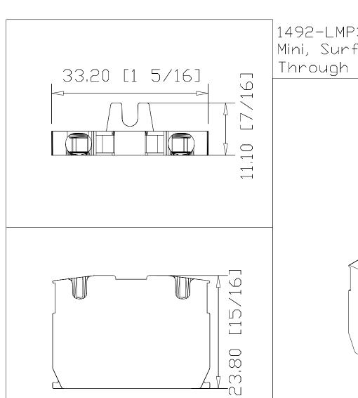
1492-LMP3E Mini, Surface Mount, Feed-Through End Terminal Block
