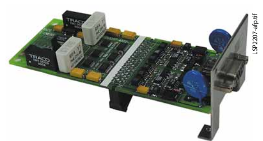
Fig. 6/22 Fiber-optic Ethernet communication module for IEC 61850 with integrated Ethernet switch
