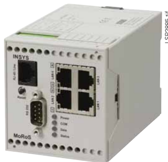
Fig. 13/75 7XV5820 Modem-Router-Switch (MoRoS)
