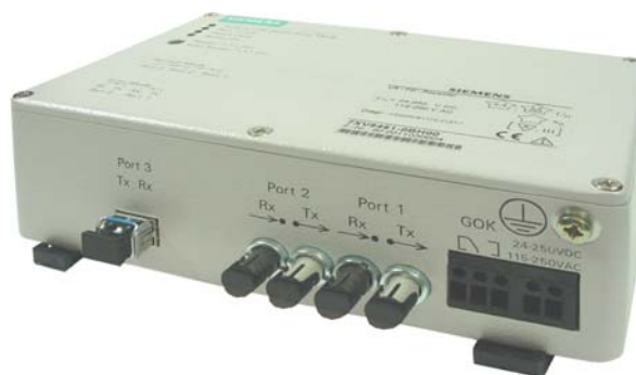
Fig.: Optical repeater with wide-range power supply
