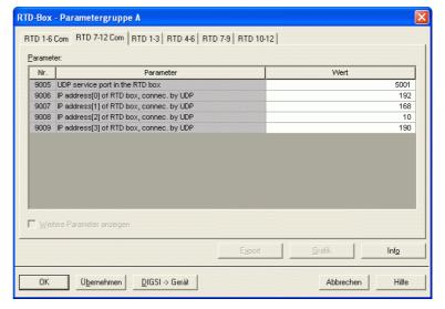
In the next step all required sensor inputs are configured. Depending on the application, 3 RTD inputs each are available in one page.
