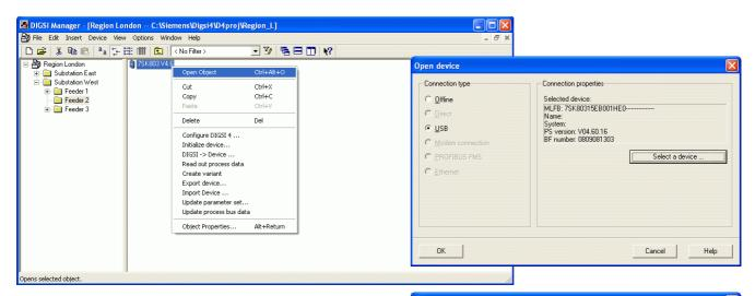
In the window "Open device" the device may be selected with "Connection type" – "USB", or the connection can be directly established through "Ethernet".
