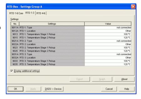
First, the "**Type**" of the sensor, e.g. Pt 100 Ohm, is selected for "**RTD 1**".
