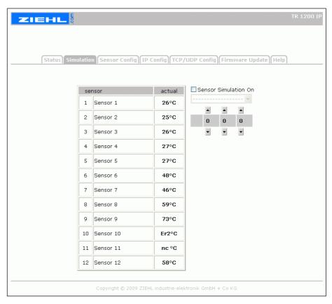
If this is unwanted the check mark "**Sensor Simulation On**" has to be removed. After approximately 3 seconds the real (actual) measured values of all sensors will be displayed and transferred to the protection device.
