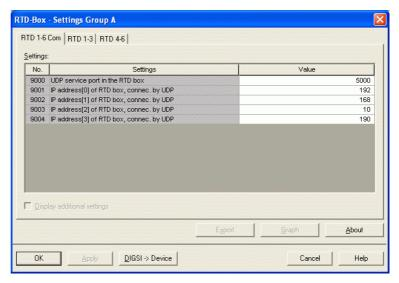
If "Ext. Temperature Input Connection Type" "12 RTD Ethernet" was selected, the first set of settings will be entered under "RTD 1-6 Com".
