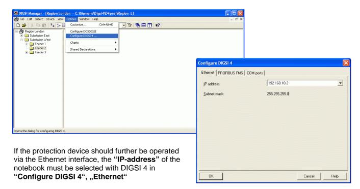
**NOTE:** From DIGSI 4.82, the IP addresses of all the available Ethernet interfaces of the PC/notebooks are available for selection in the pull-down menu.
