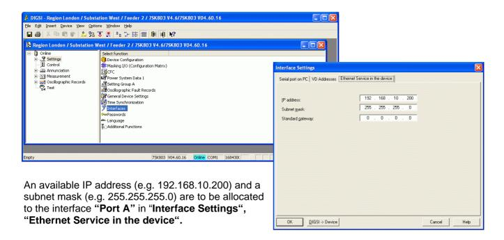
Save in the protection device with "DIGSI -> Device"
