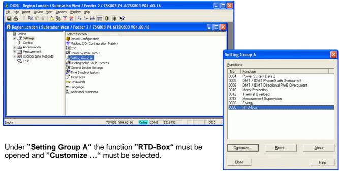
In the following section the protection device will get the UDP-Serviceport and the IP-Address of the RTD box. Through this address/port the protection device will later retrieve the temperature values.
