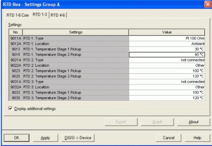
When all measuring inputs have been configured, the settings are transferred to the protection device through the button "DIGSI -> Device".
