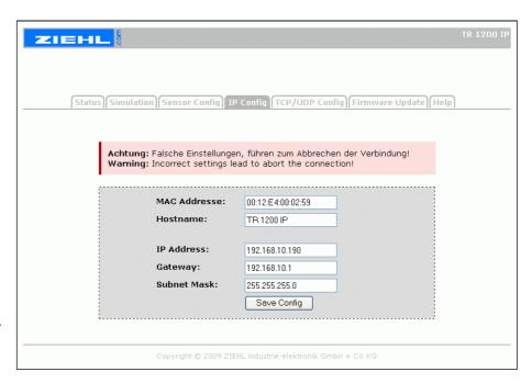
Save the settings with "Save Config". Then the Web-Browser has to be re-started with the new IP-Address.
