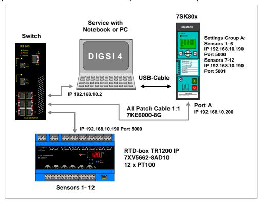
**Note:** The network must be restricted to those devices that are directly communicating with the RTD box TR1200 IP or communicate with the protection devices through DIGSI 4.
