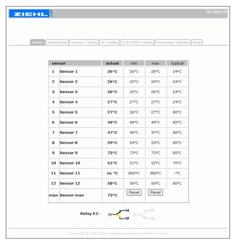
**Note:** The "high" temperature values (860/980°C) shown on the unconnected sensor inputs (e.g. sensor input 11 "nc °C") are "status alarms". They will not be evaluated in the protection device.
