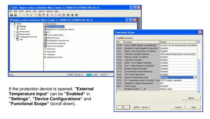
The default value for "Ext. Temperature Input Connection Type" is "6 RTD simplex operation". It has to be changed accordingly.
