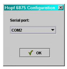
After selecting the appropriate interface the **hopf** 6875 configuration software will try to connect to the radio-controlled clock. If no connection can be made a corresponding message will appear. In this case please check that the cable is correct and/or that the cable is connected to the correct interfaces.
