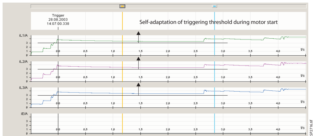
Fig. 4 Self-adaptation of triggering threshold during motor start
