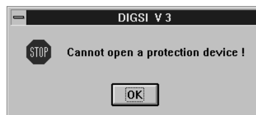
Fig. 4/27 Message if no protection devices are present
