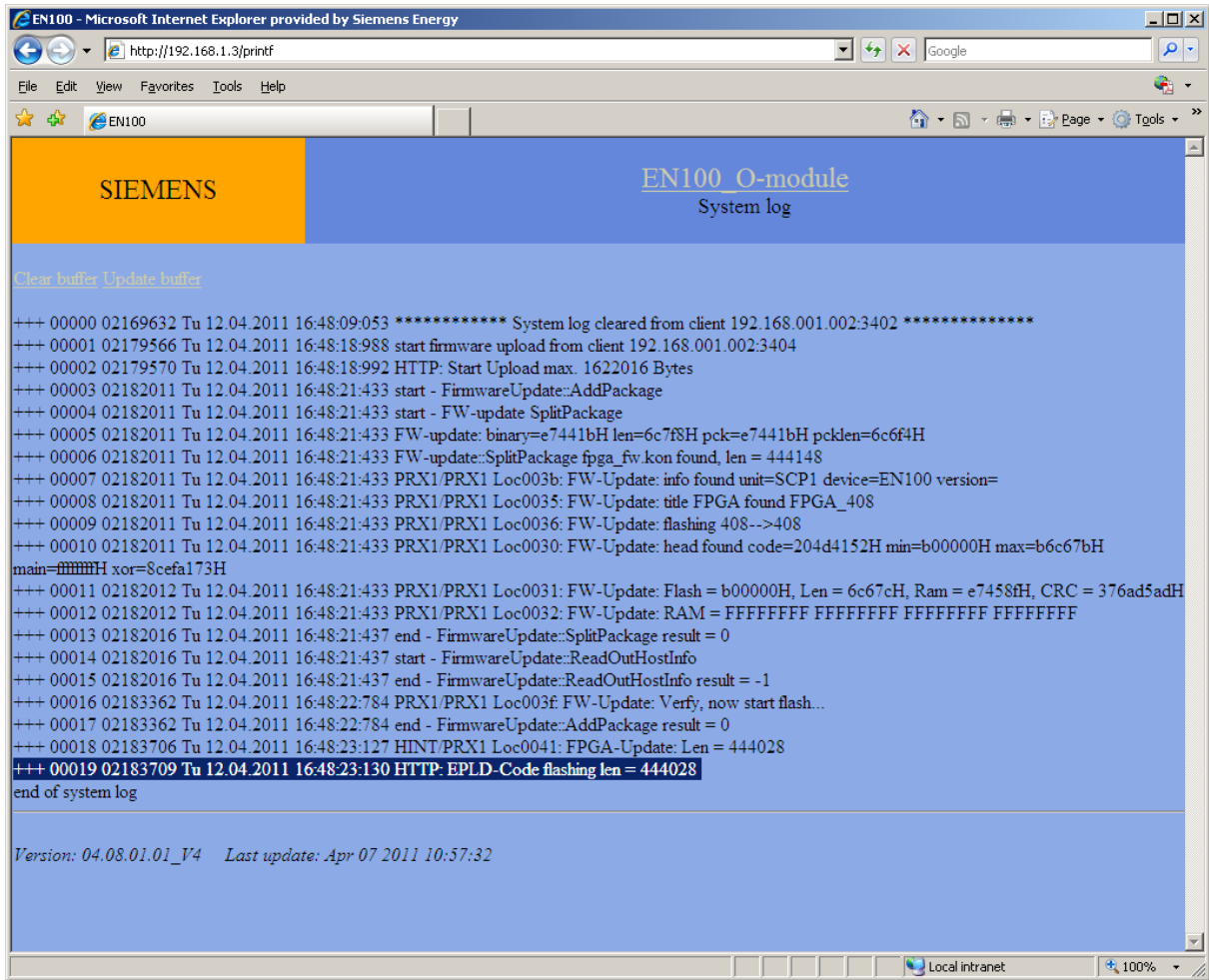
Figure 4-14 - Flash check in system log
