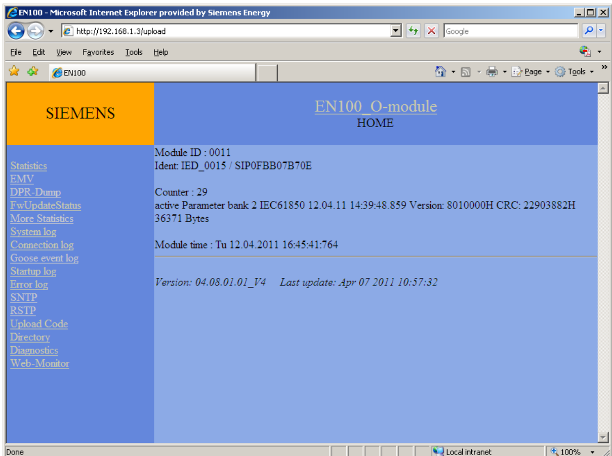
Figure 5-9 – Module home page after failed download of a wrong binary file
