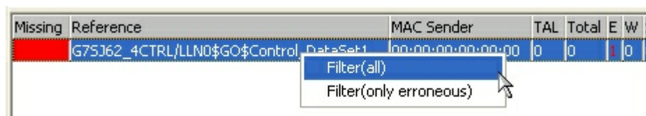
Figure 17: Marking a GOOSE and setting a filter by clicking with the right mouse button
