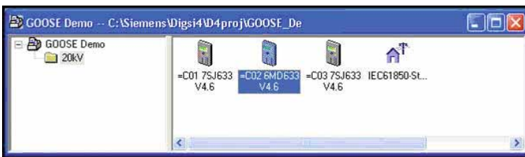
Fig. 4 "IEC 61850 substation" icon in the DIGSI 4 manager
