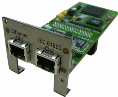
Double the pleasure: The physical interfaces of the EN100 are there twice
