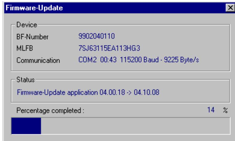
Two components are being loaded one after the other: the bootsystem and the firmware itself (application). When you load a firmware for an active communication module than no bootsystem will be loaded.
