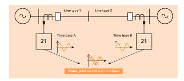
Viewing fault records of parallel lines at the same time requires only a few mouse clicks. A cursor adjusts all records to a common time base (characteristic position). The "Synchronize Fault Record" function shifts both fault records in such a way that the cursors fall on one instant. Then, comprehensive system-wide fault analysis involving more than just one relay has become feasible.
