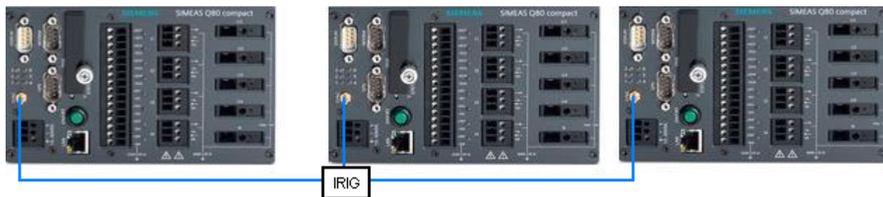
Example for synchronization with IRIG-B for stand alone devices
