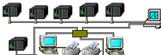
Example of a complex network with PCs and multiple SIMEAS Q80 7KG8080
