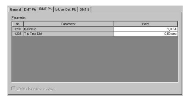
It will be defined an inverse curve with three parameters ( $I_n$ ,  $T_p$ , type of curve). The inverse curve stage generates a trip signal throughout the whole current area, but with the beginning from the intercept point the definite time ( $I_p$ ,  $I_p$ ) protection trip times are shorter and the definite time stages will lead to a final trip first.
