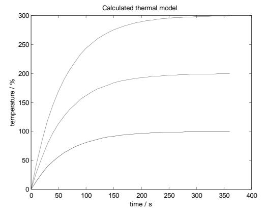
The upper diagram shows us the temperature behaviour in case of three different incoming currents. Higher currents reach the 100% temperature faster. In the first part the temperature rise is similar to a simple linear equation  $y = k \cdot x$ .
