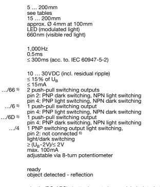
plastic (PC-ABS); 1 attachment sleeve, nickel-plated steel plastic (PMMA) with connector: 10g with 200mm cable and connector: 20g with 2m cable: 50g2m cable (cross section 4x0.20mm<sup>2</sup>), connector M8 metal, 0.2m cable with connector M8 or M12
