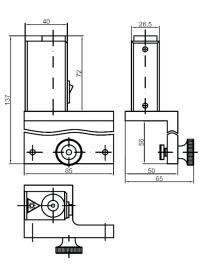
Laser Alignment Aid LA-78UDC Mounting: UDC
