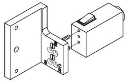
Fixing with countersunk screws included.
