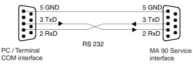
Connecting the service interface of MA 90 with a PC or terminal
