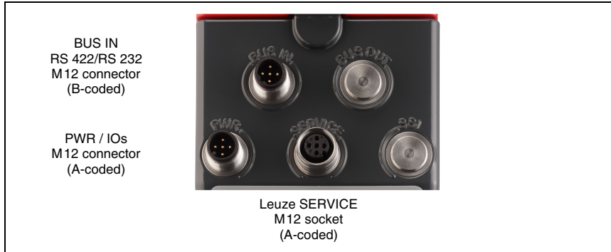
Figure 7.1: Connections of the AMS 300 i
