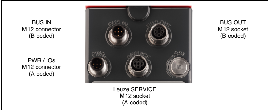
Figure 7.1: Connections of the AMS 301 i
