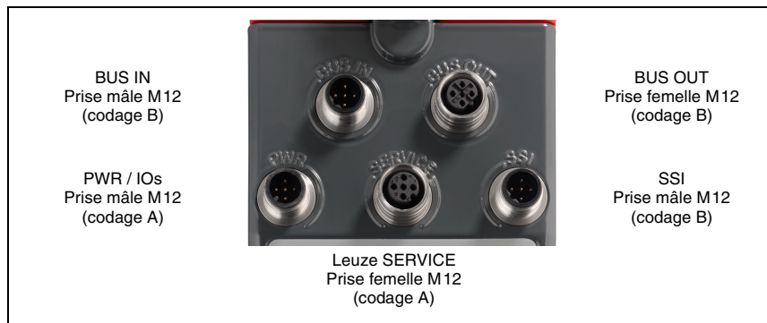
Figure 7.1 : Raccordements de l'AMS 304 i
