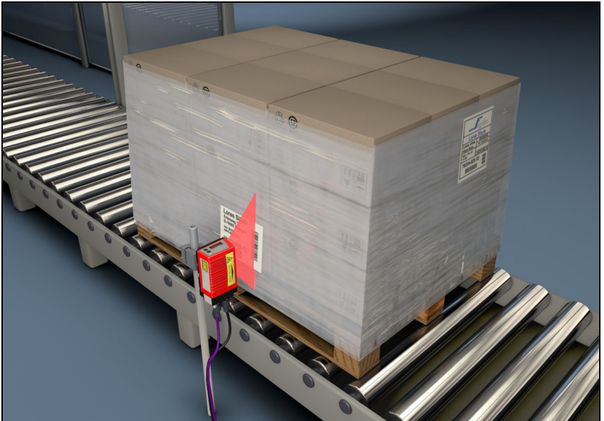
Figure 4.8: Deflection principle for the line scanner
