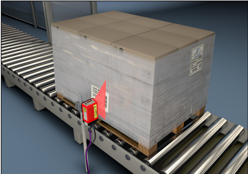
Figure 4.8: Deflection principle for the line scanner
