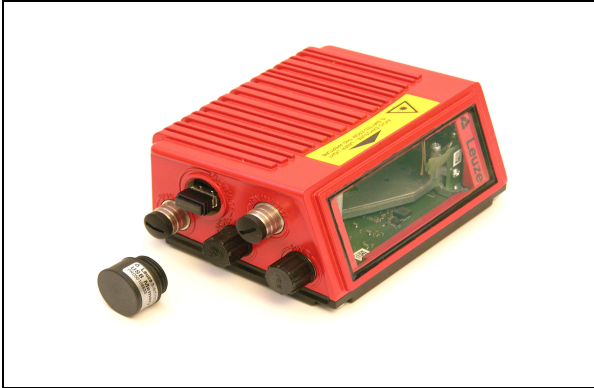
Figure 10.19: Installing the external parameter memory
