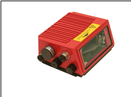
Figure 10.20: BCL 558 i with installed parameter memory
