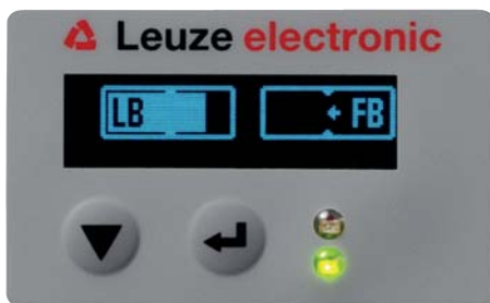
Figure 8.1: Example: display showing an incorrectly aligned light curtain
