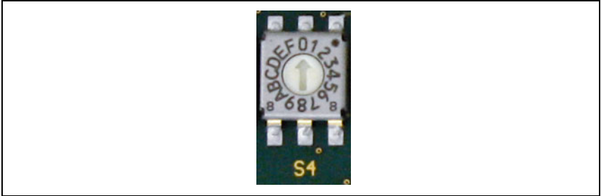
Figure 8.5: Rotary switch for device selection
