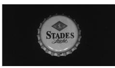
Figure 4.36: Inclined camera alignment with only three illumination quadrants active (reflected quadrant is off) nearly all reflections in the image are suppressed
