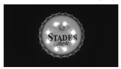
Figure 4.34: Vertical camera alignment - maximum reflections
