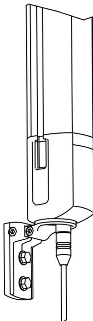
Figure 6.14: Support pivotant BT-240C
