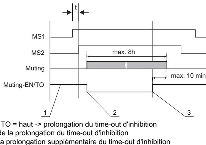
Figure 4.6: Prolongation du time-out d'inhibition
