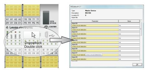
Figure 4-9 Opening the device parameterization editor for all I/Os
