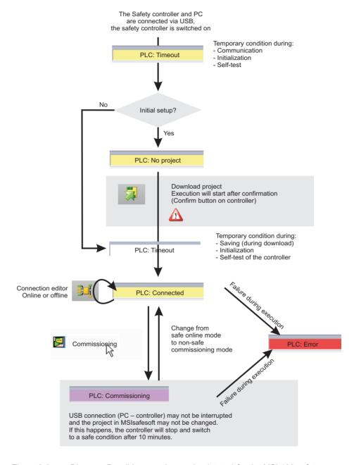
Figure 3-3 Diagram: Possible operating modes (status) for the MSI 100 safety controller
