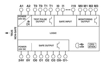
Figure 3-2 Block diagram for the MSI 100 safety controller
