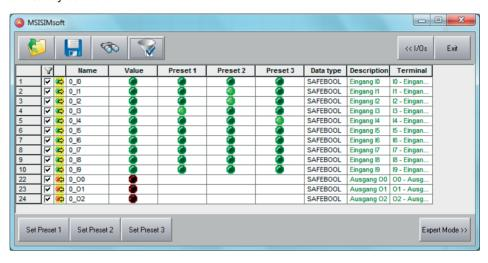
Figure 4-16 Simulation of the safety controller in MSIsafesoft
