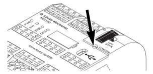
Figure 5-6 Confirming the configuration with the "Confirm" button
