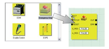
Figure 4-4 Inserting safe functional blocks and functions from the toolbox in the connection editor
