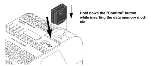
Figure 5-7 Pressing the "Confirm" button while inserting the data memory module
