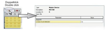
Figure 4-10 Opening the device parameterization editor for one specific I/O
