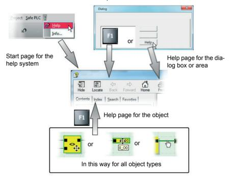
Figure 1-1 Calling the online help in the MSIsafesoft configuration software
