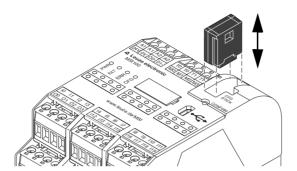
Figure 3-8 Data memory module AC-MSI-CFG1 on the MSI 100
