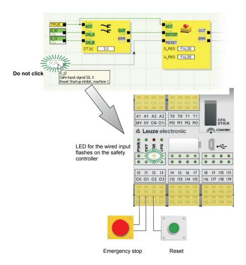
Figure 2-7 Simplified schematic view: Wiring check
