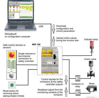
Figure 2-1 Typical structure of a safety system with MSI 100
