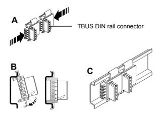
Figure 3-9 Mounting TBUS DIN rail connectors
