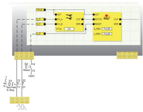
Figure 2-4 Implementing cross-circuit detection for an emergency stop control device at inputs I0 and I1 of the safety controller
