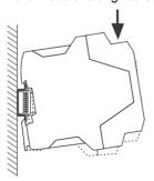
Figure 3-10 Attaching the MSI 100 safety controller to the DIN rail
