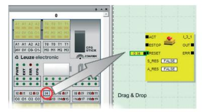
Figure 4-6 Inserting a signal in the connection editor
