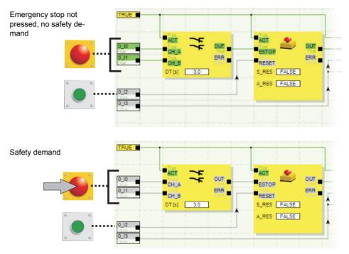
Figure 5-8 Example of a function test for the safety system using MSIsafesoft online mode
