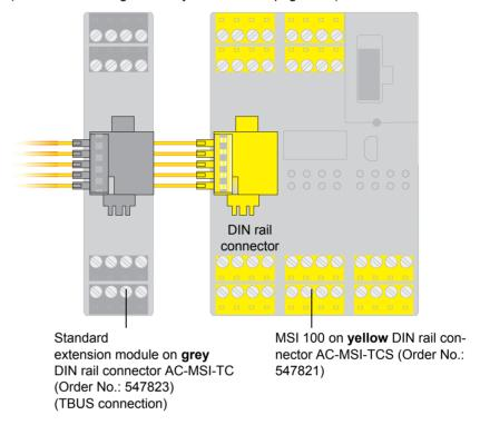
Figure 2-2 TBUS DIN rail connector from Leuze electronic
