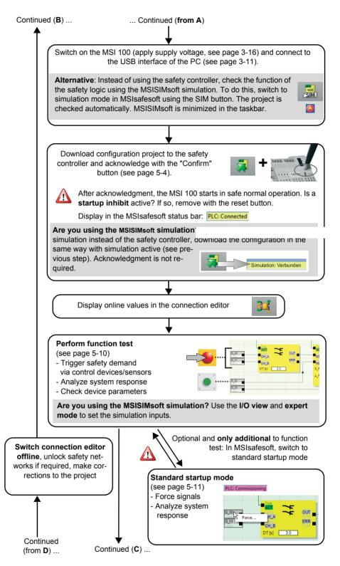
Figure 5-2 Flowchart: Configuration from A to Z (2 of 3)
