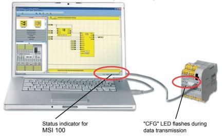
Figure 5-4 USB connection between PC and safety controller
