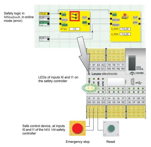
Figure 2-6 Simplified schematic view: Hardware diagnostics in the event of an error at a safe functional block
