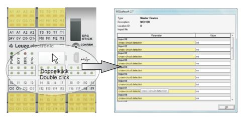
Figure 2-5 Parameterizing cross-circuit detection for a module input
