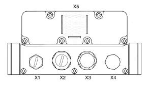
X1 Restart button connection X2 PROFIBUS output cable X3 PROFIBUS input cable X4Power supply X5 Optical PC interface
