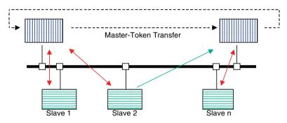
Bild 2.1-1: The functional principle of PROFIBUS
