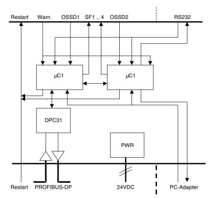
Bild 2.4-1: Design of the PROFIsafe adapter
