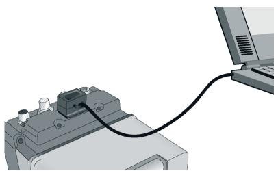
Bild 4.3-2: Connecting PC and RS4/PROFIsafe with optical PC adapter
