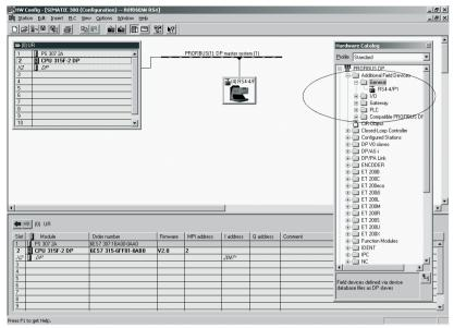
Bild 6.1-1: Hardware configuration by means of STEP 7
