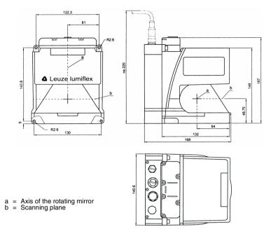
Bild 9.0-1: Dimensional drawing RS4/PROFIsafe
