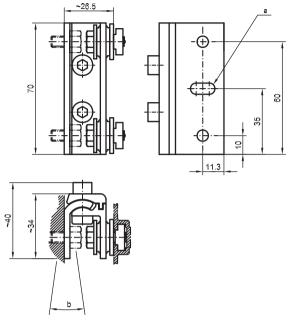
Picture 8.3:Option: Swiveling mounting bracket with shock absorber
