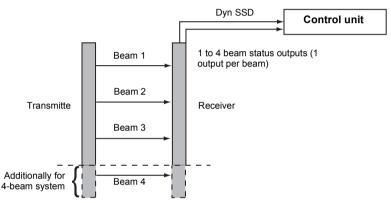
Picture 3.1:Working principle of the opto-electronic protective device
