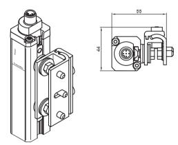
Picture 5.5:Swiveling bracket with shock absorber
