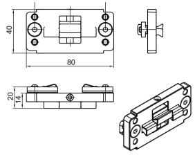
Picture 5.4:Clamping bracket for C-slot mounting
