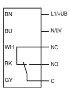
The relay-functions "NC" and "NO" bear on the switching mode "Dark-ON".
